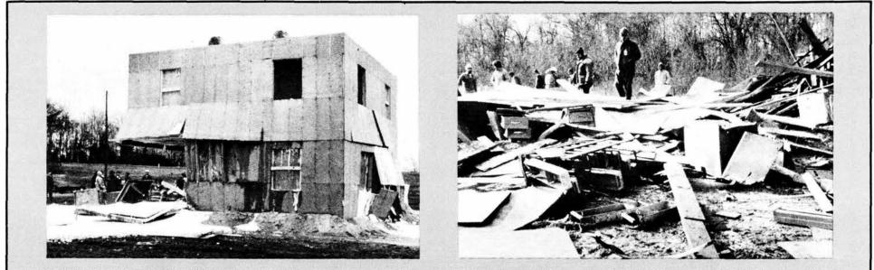
DRAMATIC BLAST MITIGATION effect of aqueous foam is illustrated in these two photos taken during a joint study by Sandia's Special Projects Division 5256 and the Naval Tech Center's Explosive Ordnance Disposal group at Indianhead, Maryland. In the photo at left, a two-story frame test structure was filled with aqueous foam, then 15 lbs. of C4
